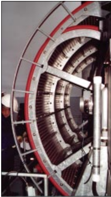
Wampfler: a level wind reel on a crane in the Port of Århus (left) and (right) the company's Cobra energy chain as installed on 15 Noell RTGs just delivered to DP World's Centerm, Vancouver, BC terminal
