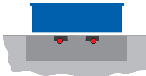
Cable installed directly into the floor
